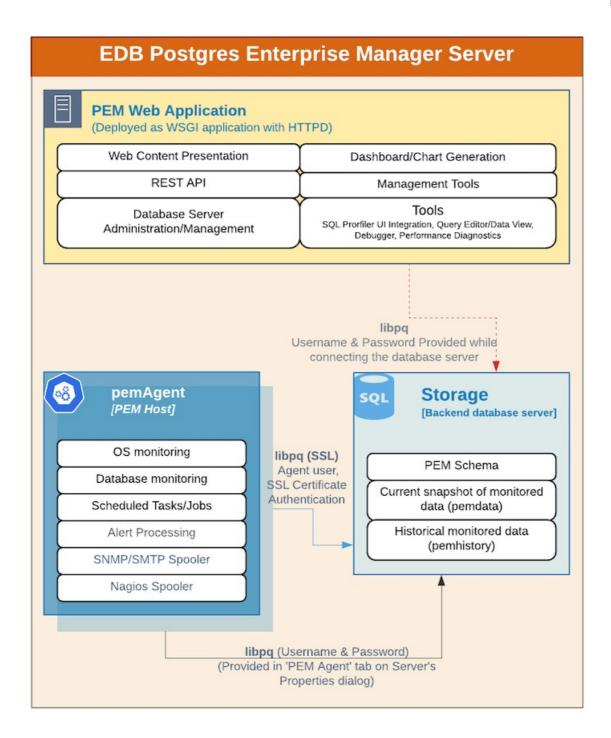
The PEM server consists of an instance of Postgres, an instance of the Apache web server providing web services to the client, and a PEM Agent. PEM uses a server-side cryptographic plugin to generate authentication certificates.
