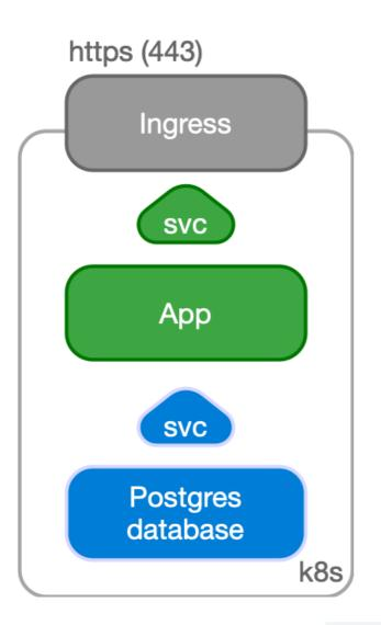
The application, normally stateless, is managed as a standard Deployment, with multiple replicas spread over different Kubernetes node, and internally exposed through a ClusterIP service.
