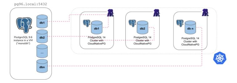
For example, the YAML below creates a new 3 instance PostgreSQL cluster (latest available major version at the time the operator was released) called cluster-microservice that imports the angus database from the cluster-pg96 cluster (with the unsupported PostgreSQL 9.6), by connecting to the postgres database using the postgres user, via the password stored in the cluster-pg96-superuser secret.
